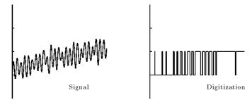
If the digitized signal is put through a resistor-capacitor circuit to smooth it out, some reasonable approximation to the original signal can be recovered. There is no theoretical limit to the accuracy possible with this method, as long as the sampling rate is high enough.
