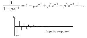
Filters are usually designed in such a way that the output  $g(n\Delta t)$  depends linearly on  $f((n-m)\Delta t)$  for a finite set of values of  $m \ge 0$  and on  $g((n-m)\Delta t)$  for a finite set of values of m > 0. For such a filter, the z-transform of the impulse response is a rational function of z, which means that it is a ratio of two polynomials
