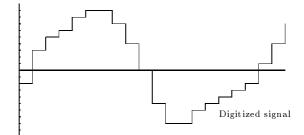
This part of the process of turning an analog signal into a digital signal does entail some loss of information, even if the original signal contains no frequency component above half the sample rate. To see this, think what happens to a very low level signal. It will simply get reported as zero. There is a method for overcoming this limitation to a certain extent, called *dithering*, and it is described in  $\S7.2$ .
