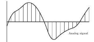
Next we have the sampled signal, but still with continuously variable amplitudes.
