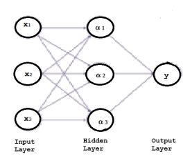
Scheme of a perceptron in the case n = dim(x) = 3.
