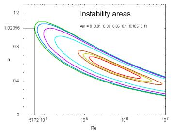
Critical curves in the plane of the wave number a and Reynolds number Re at different applied magnetic field, for a large value of the magnetic Reynolds number (Rm = 1).
