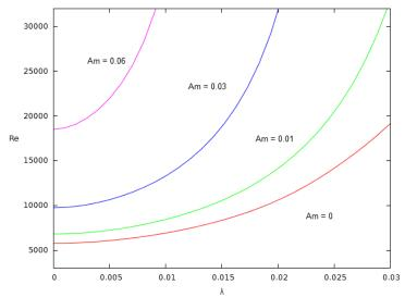
Stabilizing effect of finite slip length  $\lambda$  at different magnetic fields (with Rm = 1).
