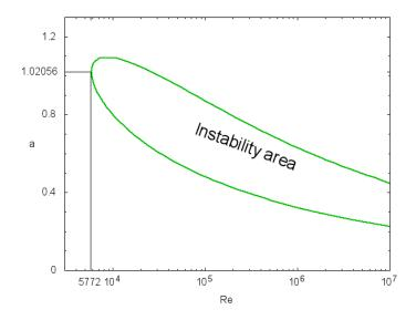
Critical curve in the plane of the wave number *a* and Reynolds number *Re*.
